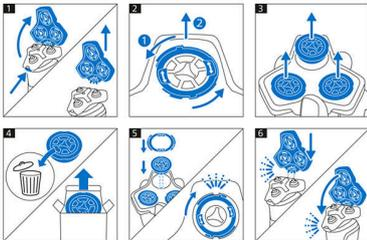
1. Press the release buttons and detach the shaving head holder. 2. Turn the retaining rings counterclockwise and remove them. 3. Remove
